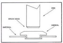
UNISEAL was designed for pipes of standard outside diameter (SCH 40). The tapered inner diameter forces the outer diameter to expand and securely seal the penetrating pipe/tubing without adhesive hardware or threads. It will seal for any flat or curved material even if the pipe is at an angle as great as 15°.
